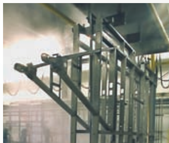
Frames are protected from corrosion by the 12-stage E-Coat™ finishing system.
